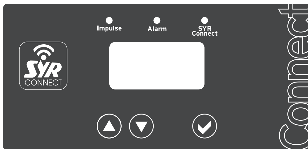
Fig. 12: User interface with display, LED and control buttons
